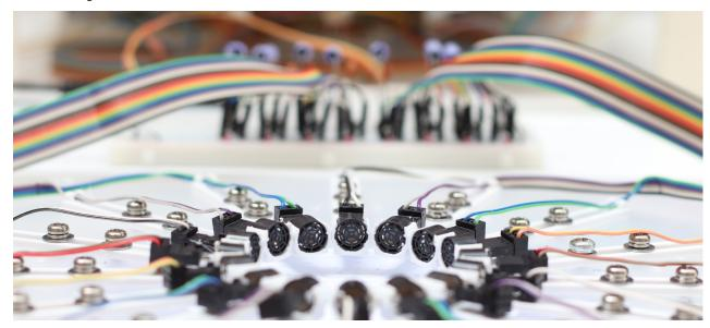
Fig. 16: Transducer array and driving circuit.
