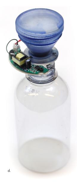
Fig 4: a-c: square, hexagonal, and 16-sided transducer array plates with 3D printed transducer mounts. d: The atomiser assembly to be held above the transducer array for creating fine mists of ink droplets.
