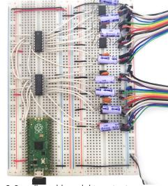
Fig. 5: Breadboard-based driver circuit.
