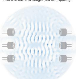
[D] Interference between adjacent transducers in a 2x3 opposing setup introduces wobble rather than making a stronger version of [A].
