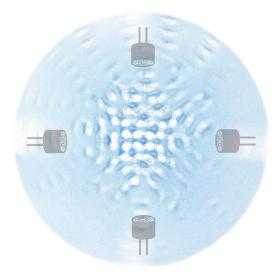
[C] When 4 inward-pointing transducers are all in phase and with equal amplitude a grid of spots immerges.
